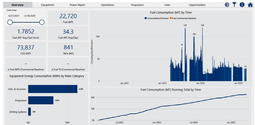
The EEI dashboard displays fuel and energy consumption, GHG and nitrogen oxide (NO x ) emissions, and helps identify areas for energy optimizations and emission reductions.
